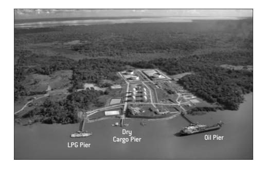
The downstream berth, near the LPG pier, is formed by the Floating Operation Platform (POF-2) and mooring buoys, has the same configuration as the upstream berth and lies 360 meters from the oil pier.
