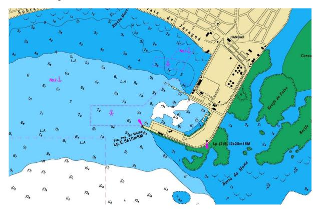
The maritime access is approximately 520 m long, 80 m wide and has a depth of about 10m to 14 m, with no entry bar. It has an evolution basin 400 m long and 360 m wide with 11 m deep.
