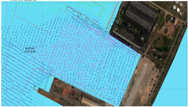
The maximum draft allowed for operations in THE PGL is 10.5 m at low tide and 11.0 m at high tide.
