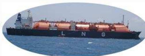
The **FSRU** is a conventional LNG vessel provided with a re-gasification plant to convert LNG into CNG, pumping it subsequently to the **TRANSPETRO** gas pipeline network. **FSRU** retain all original capabilities of a LNG vessel, however its engine will be temporarily disabled.
