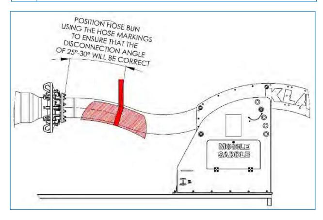
024 After correct positioning of hose bun a small amount of lift should be applied to it to take hose load away from the flange connector.
